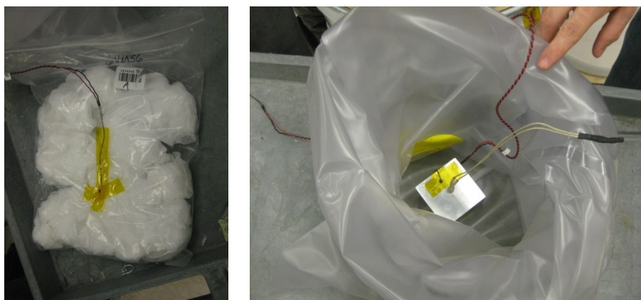
Figure 11 Thermistors on cheesecloth and aluminum block
