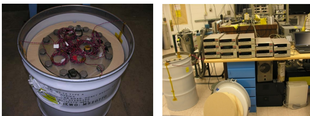
Figure 13 Testing setup, POC wired up (left) and volt meters along with MultiCal program (right)
